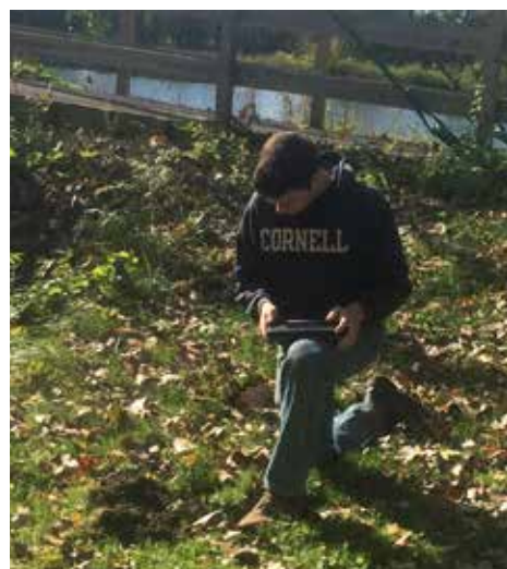
Daniel May installing a nodal recorder in Stewart Park to calibrate ground response in Ithaca Valley to seismic wave.
