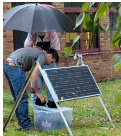
The seismograph stations installed at Ithaca High School to record the vibroseis waves as well as distance earthquakes to quantify ground response in Ithaca Valley. Professor Larry Brown observes May's work while holding an umbrella to protect them from the elements.
