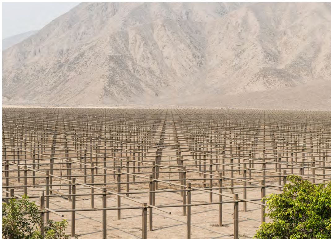
More than 18,000 dipole radio antennae help make up the Jicamarca Observatory in Lima, Peru. / Alastair Philip Wiper.
