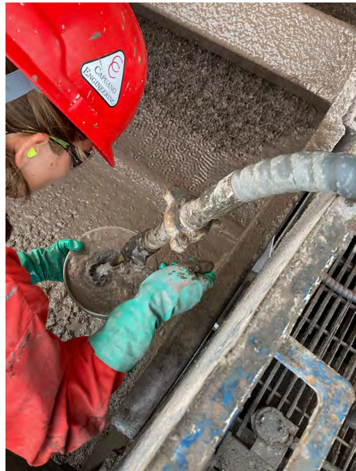
EAS undergraduate Madeline Fresonke demonstrates the messy work of catching and cleaning samples of cuttings immediately after the borehole mud carries them out of the borehole.
